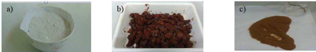
Fig 1. Wastes used in sand manufacturing : a) Ash biomass; b) Flux sludge; c) Bagasse
